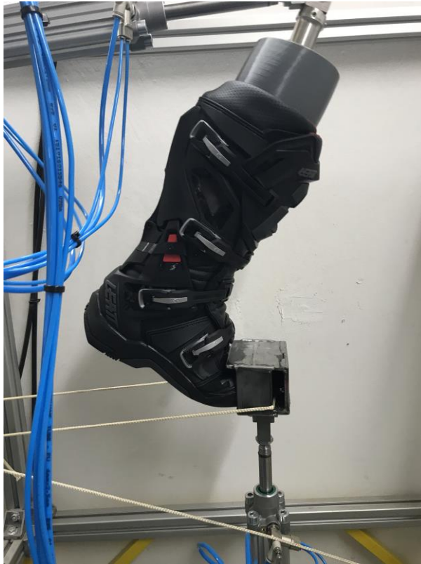
Figure 4-18: Boot fatigue testing setup
