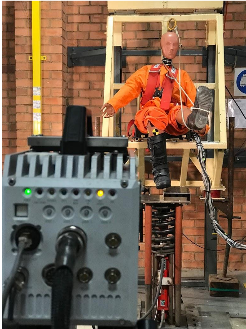
Figure 4-12: A stepped impact test with Leatt® GPX 5.5 MX Boot
