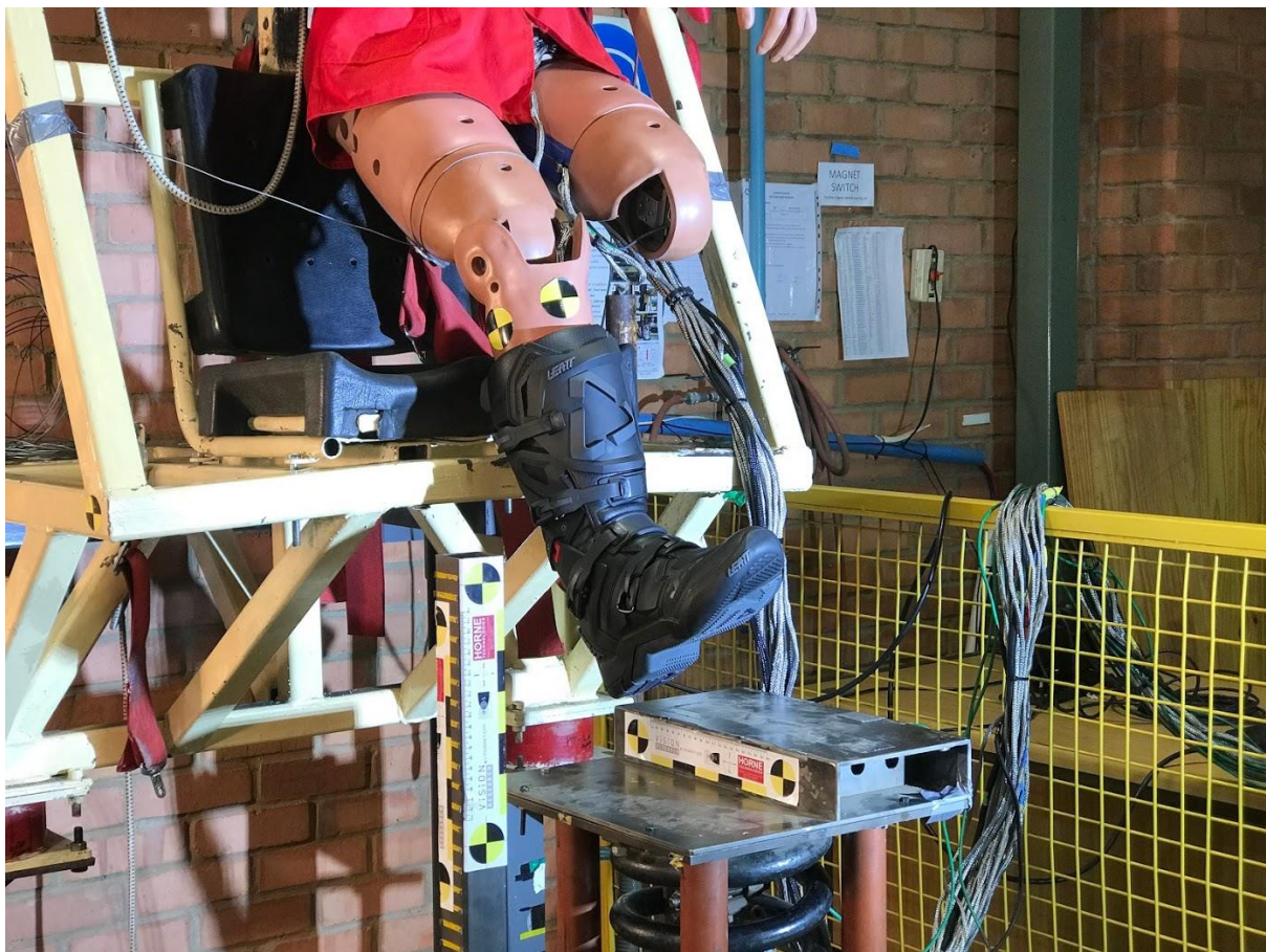
Figure 4-13: Test setup used for Knee analysis
